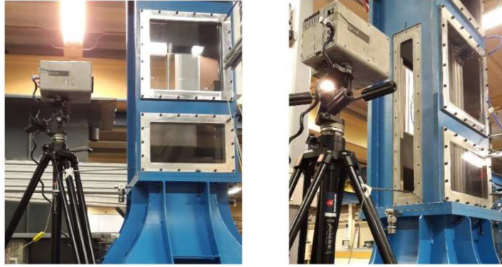
Figure 3.5: Infra-red camera measurements.
