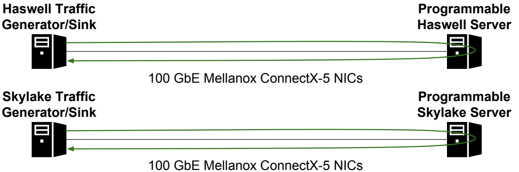
(b) Deployment at 100 Gbps using two (Haswell or SkyLake) servers connected back-to-back, each with one 100 GbE Mellanox ConnectX-5 MT27800 [73] NIC.
