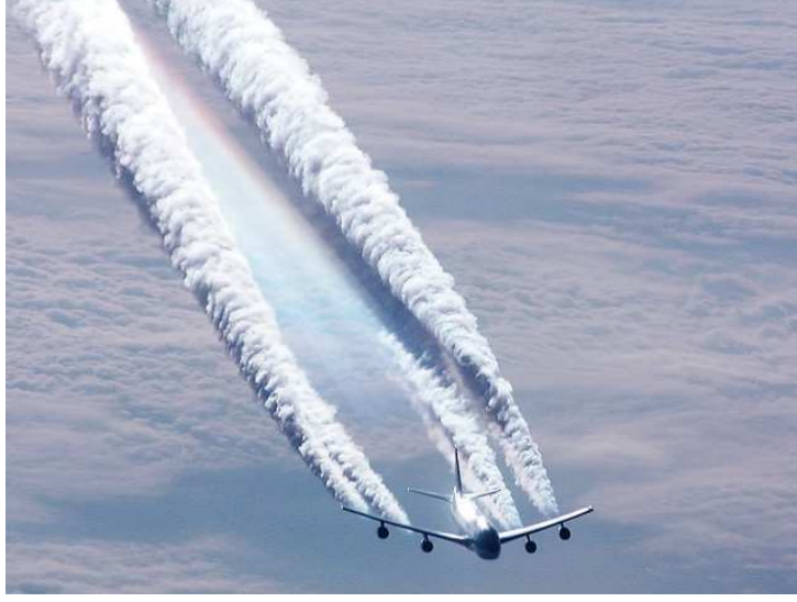
Figure 1.1: Condensation trail of a Boeing 747: the condensation trail is absorbed by the wake of the airplane and the wake vortices are clearly visible. Image taken from https://kitskinny.wordpress.com/2013/07/09/jets-clouds-effects/
