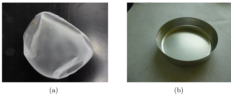
Figure 4.10 – PEO 400k films with different LiClO 4 concentrations obtained by evaporation of a DMF solution:
