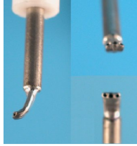
Figure 4.9.: The miniature three-hole probe used for the determination of the radial distributions of the velocity, flow angle and static pressure
