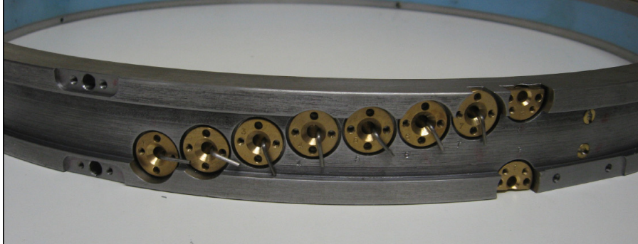
Figure 5.4.: Brass inserts including the Kulites mounted inside the casing
