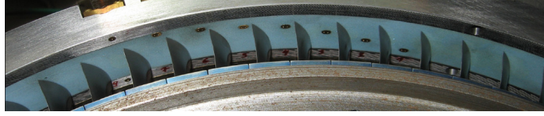
Figure 5.8.: Photograph of casing with static pressure measurement sensors
