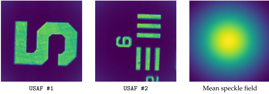
Figure 8.8 Estimates of USAF ground truth. Images of standard USAF transmission target. They are estimated using the first channel of the imaging system (see Figure 8.7). The CCD sensor acquires M images of the product between a speckle and density map f . Their average divided by the mean speckle field (Gaussian fit estimated from the M light patterns) leads to the estimated ground truths.
