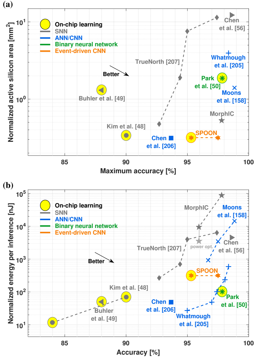
Fig. 4.8 Analysis of tradeoffs between accuracy, area and energy per classification on the MNIST dataset for SNNs, BNNs, ANNs and CNNs. Although MorphIC and the chip from Chen et al. embed online learning, the MNIST experiments of these two chips were obtained with offline-learned weights. All chips are digital and allow for technology normalization, except the design from Buhler et al. which is mixed-signal [49]. (a) Area-accuracy tradeoff. Silicon area (excluding pads) has been normalized to a 28-nm technology node using the node factor (e.g., a (28/65)^2 -fold reduction for normalizing 65nm to 28nm), except for the 10-nm FinFET node from Chen et al. [56] where data from [120] was used for normalization. The TrueNorth area varies as Esser et al. used different numbers of cores for their experiments (5, 20, 80 and 120 cores, in the order of increasing accuracy) [207]. A 1920-core configuration is also reported in [207], leading to a 99.42-% accuracy on MNIST with TrueNorth, a record for SNNs. However, as this configuration would lead to a normalized area of 980mm 2 , we only included TrueNorth configurations whose scale are comparable with the other chips. (b) Energy-accuracy tradeoff. Energy has been normalized to a 28-nm technology node using the node factor (e.g., a (28/65) -fold reduction for normalizing 65nm to 28nm). The point shown in light gray for MorphIC is a prediction resulting from the power optimizations proposed in Table 2.4 of Section 2.3.2.
