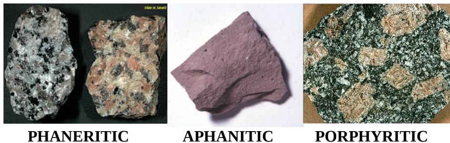
Figure 2.3. Texture of crystalline volcanic rocks.
