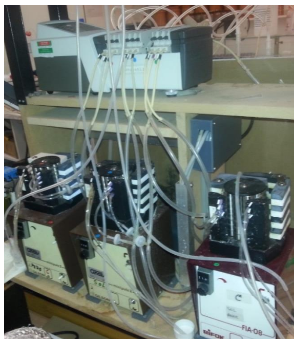
Figure 3.13. Photograph of the fluidized bed system (viewed from the back) used for volcanic rock/ash/glass dissolution (VERSION II Chapters 5 and 6)
