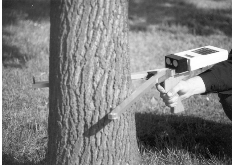
Fig. 9.2. Electronic caliper based on ultrasonics.
