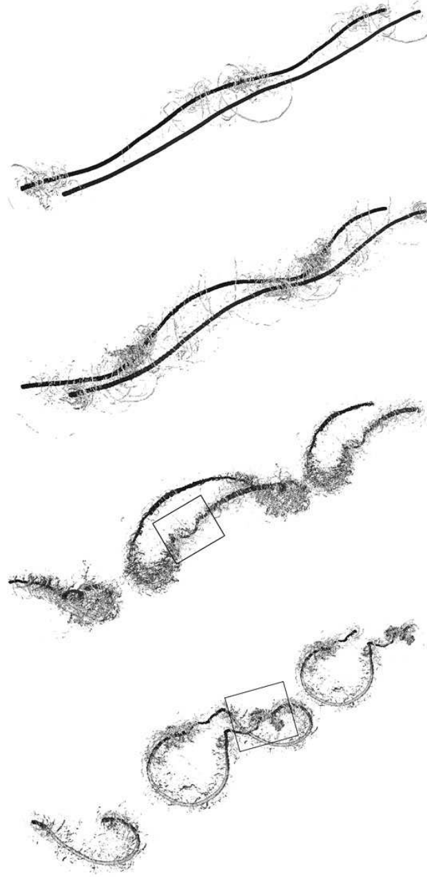
Figure 2.22: Visualization of the flow for case 0 ( N^* = 0 , \epsilon_f^* = \epsilon_1^* ), using iso- \lambda_2 surfaces colored by the axial vorticity \omega_x b_0^2/\Gamma_0 at times (from top to bottom): t^* = 3.0 , t^* = 4.0 , t^* = 5.0 and t^* = 5.5 .
