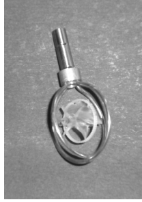
Fig. 4.8: propeller used to measure the water velocity.
