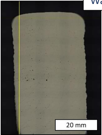
Wall 07 ER5183 with laser cleaning
