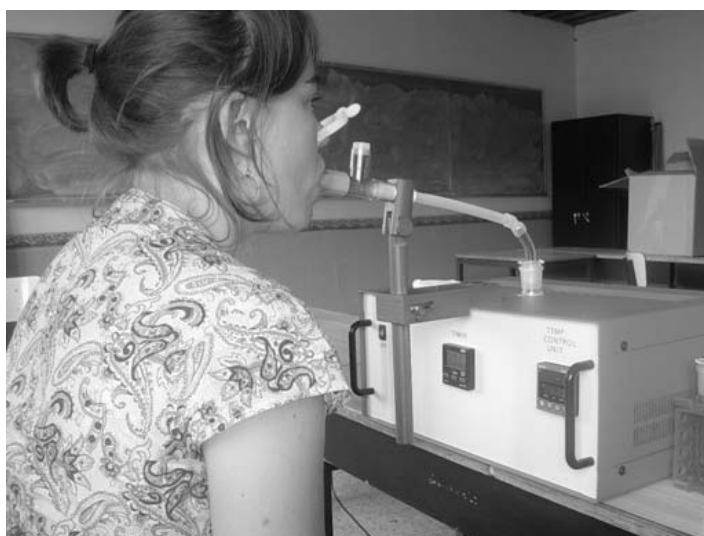
Figure 10 EBC sample collection with custom-made device.
