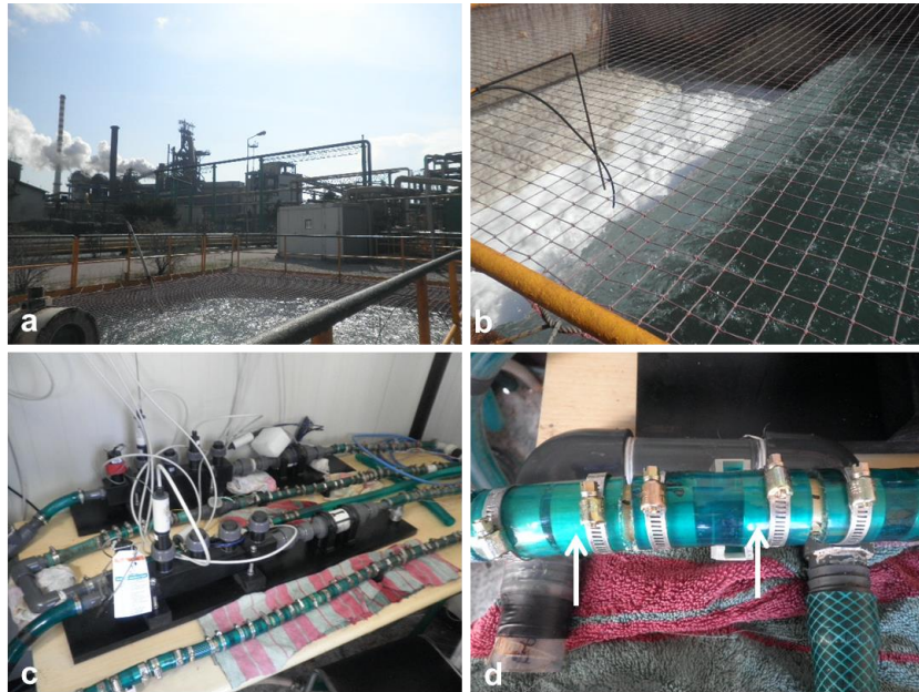
Figure 27. Pictures of field experiment: (a) power plant, (b) outlet of seawater, (c) bypass setup circulated with seawater, (d) samples (indicated by arrows) exposure in seawater.
