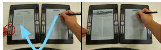
Figure 2. Conduit interaction for linked SFT. Left: With the command button pressed on the left device (red circle), tapping on a thumbnail on the right device opens the corresponding page on the left device. Right: Final result of the operation
