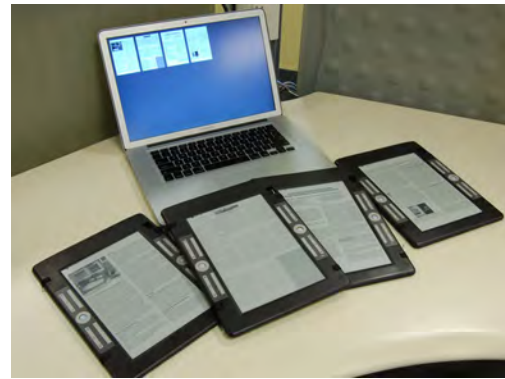
Figure 1. Sample multi-tablet setup with four tablets and a laptop computer running the remote interaction application. Note that the visualization of the tablets in the application matches the state of the tablets.
