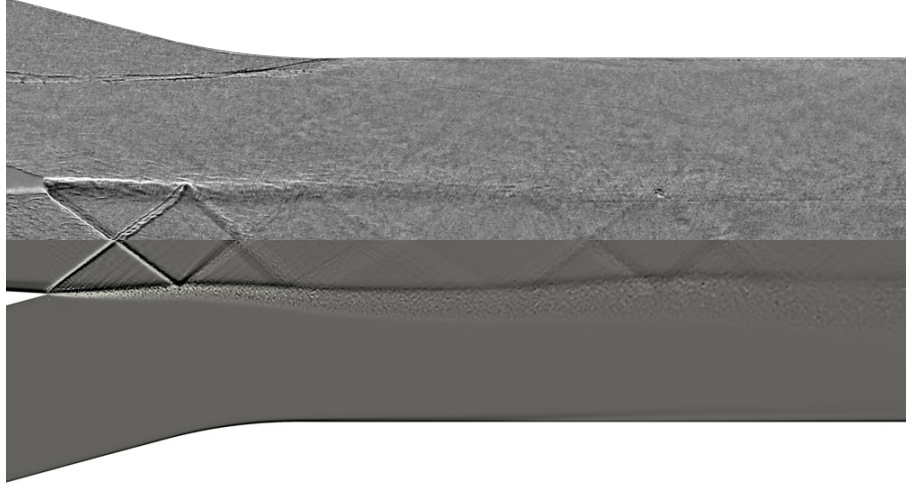
Figure 7.1: Comparison of an experimental picture obtained by shadowgraphy (top half) with the corresponding image extracted from the 3D numerical results (bottom half).
