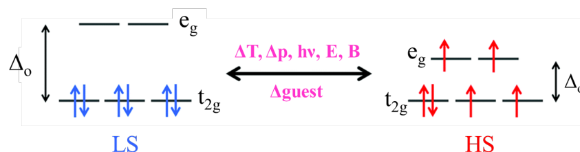
Figure 1. Schematic illustration of the d orbital splitting in an octahedral Fe(II) ion. External stimuli such as temperature, pressure, light, magnetic or electric fields and guest binding can induce spin-state switching.
