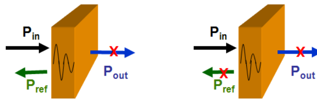
Figure 1 – Schematic diagrams for a conventional metallic shielding material (left) and for a microwave absorber (right) [3]
