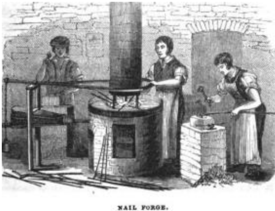
Fig. 3. Nail makers using Spencer's patent forge. THOMLINSON 1852, 37
