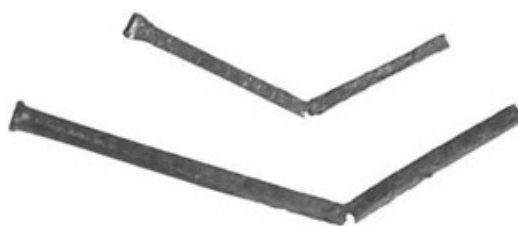
Fig. 99. Lamination 'greenstick' fractures of 1884 American cut nails. Author
