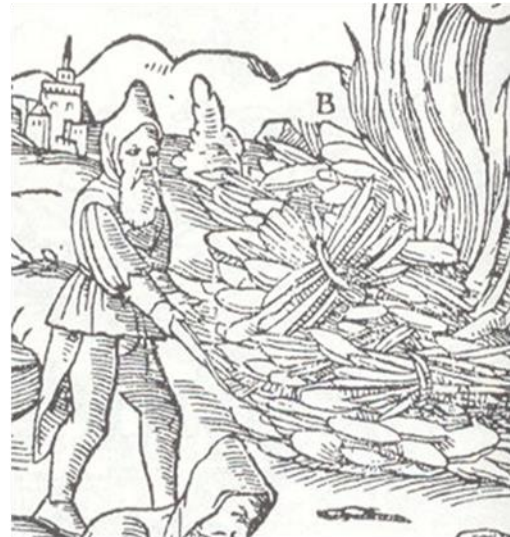
Fig.55. Breaking metal ore from rock and roasting ore on a pyre after Agricola 1556.
