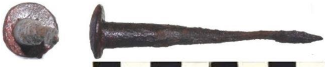
Fig. 182. An off-centre head wrought plaque nail, Courthouse, Moonee Ponds, 1888. Author.
