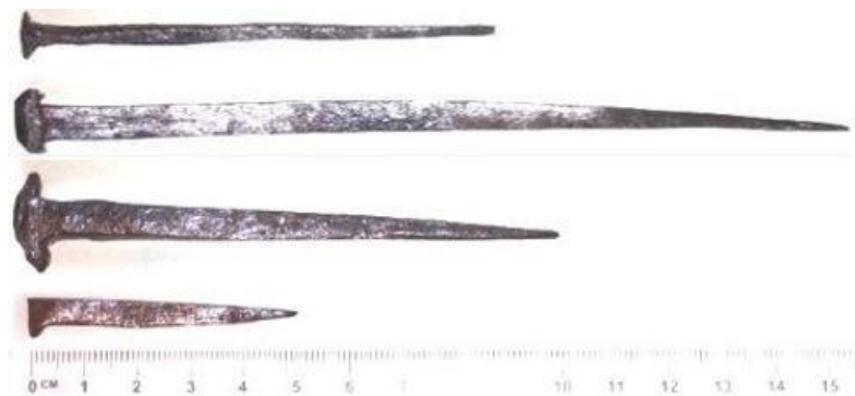
Fig. 28. Four wrought roof nails: Provence, 1795; Latvia, 1861; Somerset, 1760; & Warrnambool, Victoria, 1851. Author
