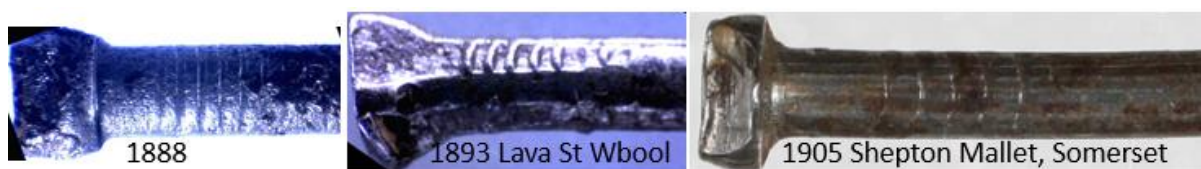
Fig. 147. Oval wire nail face clamping, diamond clamping, and head changes. Author
