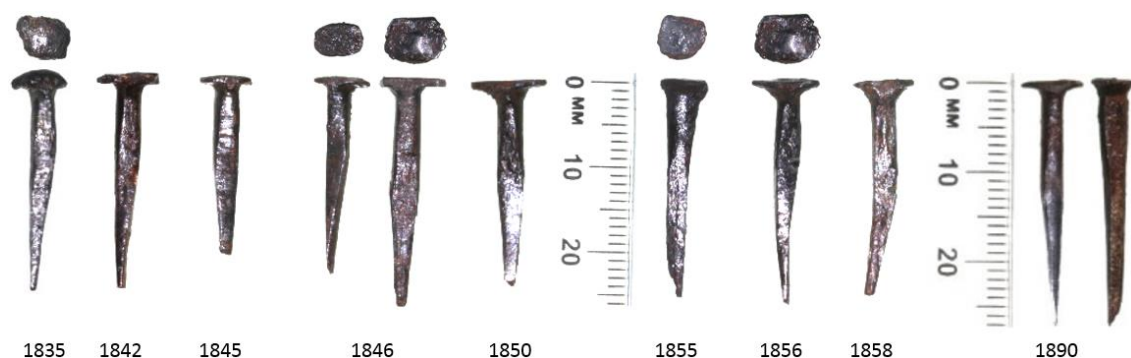
Fig. 117. Lath tack-nail found in Britain and Australia, left to right: Supreme Court Sydney, Woolmers Cottage Tasmania. Brighton UK. Two from Princes St Pt Fairy, Warrnambool, Vic. Bowlish house extension Darshill, Somerset. St Andrew’s Manse, Pt Fairy. Digby Cottage Pt Fairy, and two from Cestria, Melbourne. Author
