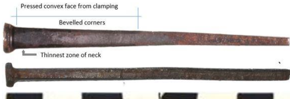
Fig. 119. American face-clamped cut nail Christ Church, Warrnambool, 1875; face view, and side view. Author
