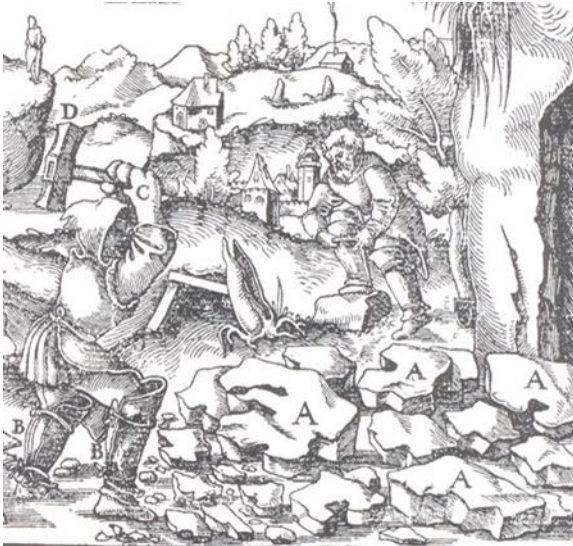
Fig.55. Breaking metal ore from rock and roasting ore on a pyre after Agricola 1556.
