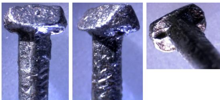
Fig. 183. Three Digi scope views of the Hobart Art Gallery 'forage cap' head wire nail, Author
