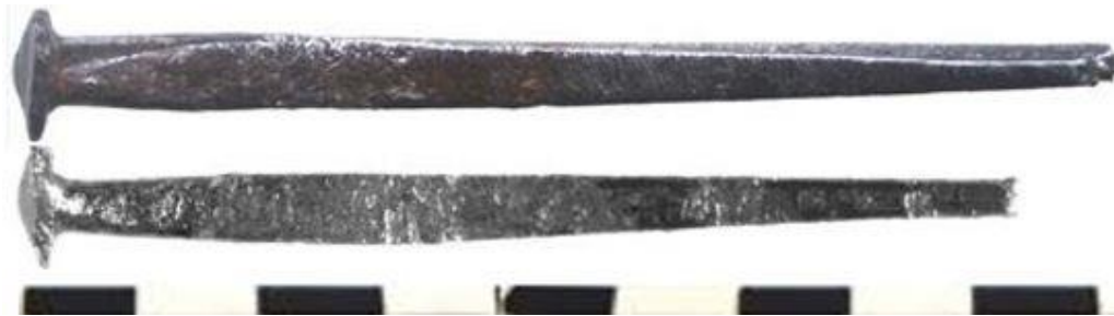
Fig. 104. British cut nails circa 1816 -1845 showing 'waists' due to side clamping below the heads. Author
