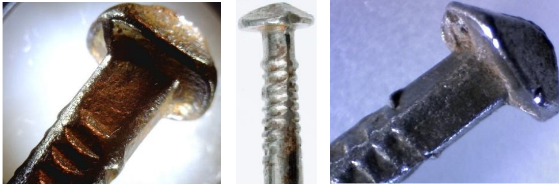
Fig. 141. Four sided clamping, 1878 with opposed clamping, concave, 1887, and diamond, 1888. Author
