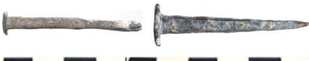
Fig.77. Galvanised wrought common, Digby cottage, Port Fairy, Victoria, 1856, and galvanised gate nail, Adelaide, South Australia, circa 1855. Author
