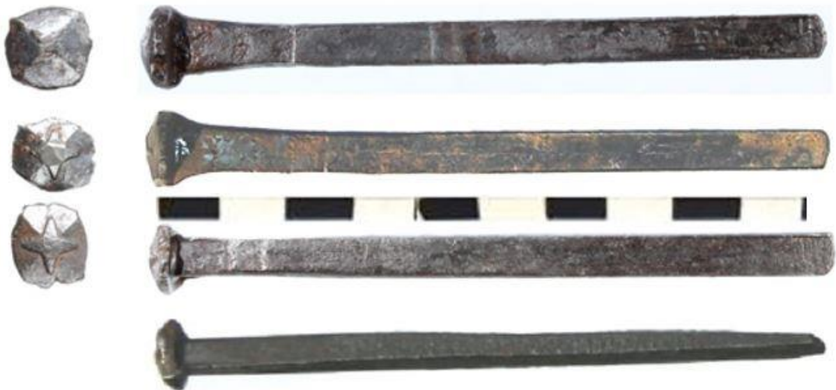
Fig. 124. Ewbank variations; 1834 model, 1869 'Starhead', and 1881 square-grip model, face and side. Author The changes to the Ewbank nail are useful in setting threshold dates, and because of its ubiquitous nature in Australian buildings, the changes are powerful determinants. One further change, already shown above in fig. 114, section 4.4.15, was the factory's introduction of a replica in cut form. This
