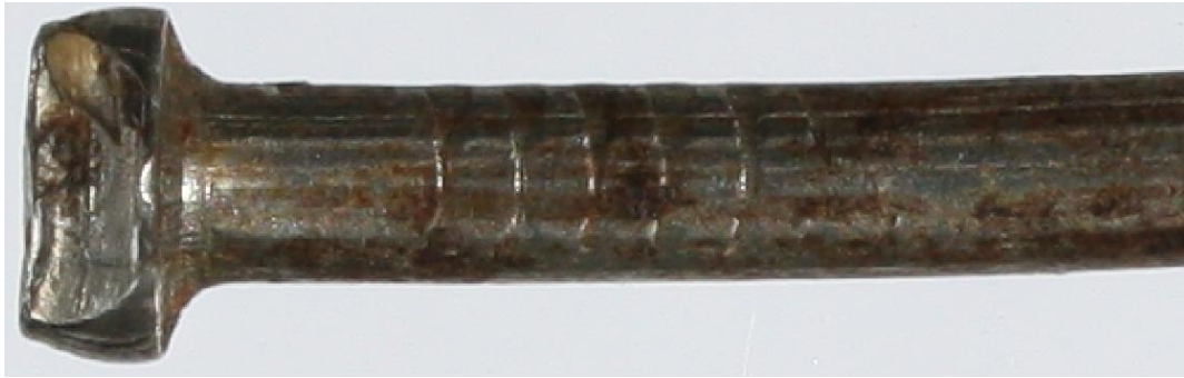
Fig. 130. Oval nail, Shepton Mallet, Somerset, 1905, showing roller marks and 'forage cap' head. Author.
