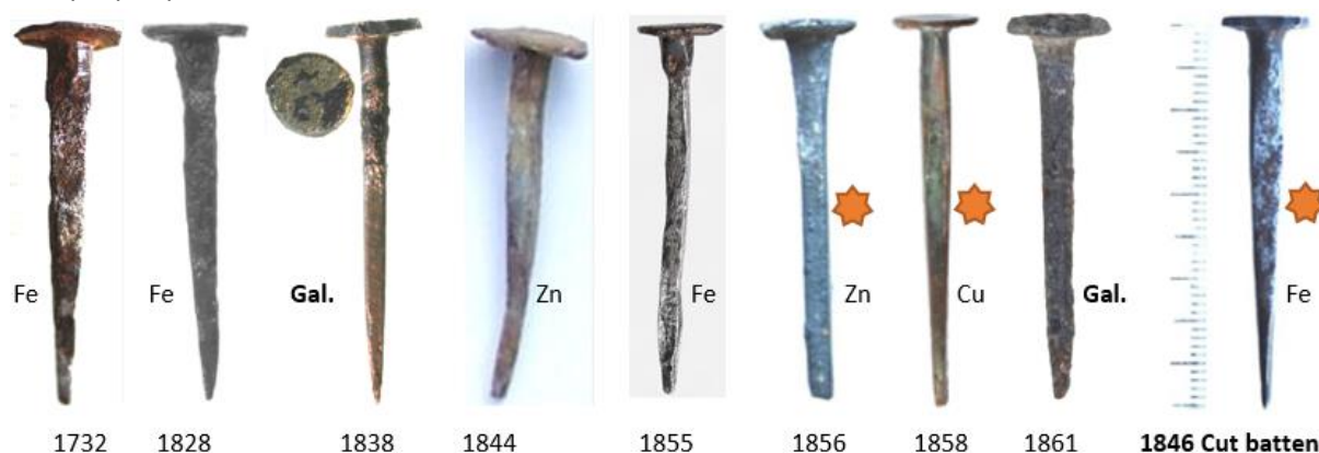
Fig. 154. The progression of slate nails and the influence of the cut nail technology. Author
