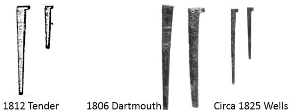
Fig. 103. Headless and spur-headed cut floor brads, 1806, Dartmouth, and joiners' brads, circa 1825.
