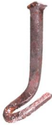
Fig. 110. British cut clasp nail, 1845, Montague Terrace, Brighton, Sussex, showing early 'wings' and significant distortion. Author.
