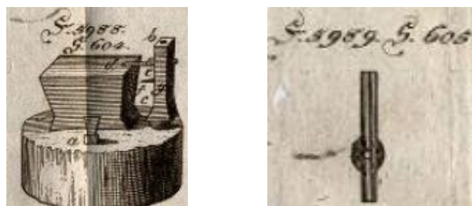
Fig. 66. The nailor's block with obore after Krünitz, Braunschweig, Date unknown
