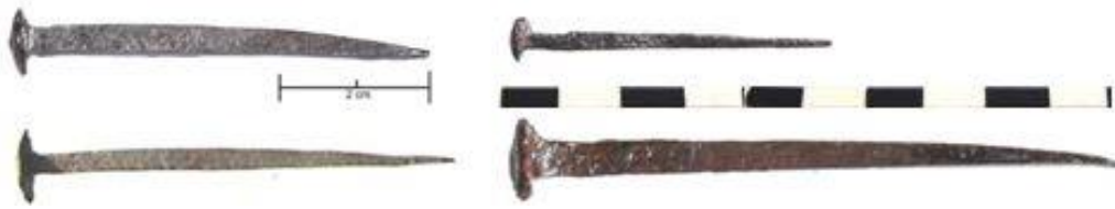
Fig.113. Rafter nail 1843, Pontville, (top left; photo Luebbbers), An 1853 Portland flat profile version, top right. A rafter nail, 1850, Warrnambool, and Princes Highway, Garvoc, 1880. Author.
