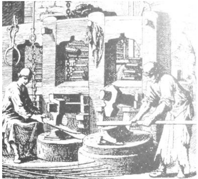
Fig. 4. Circa 1485, a method of making iron wands, seen in foreground, from flattened ribbon via the Reckhammer (on right) and the Zeinhammer on left. WEIGEL 1698, 389
