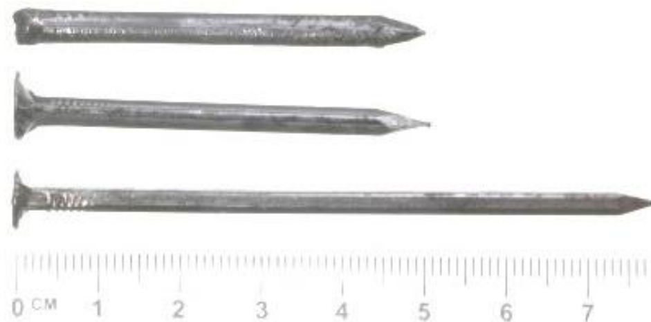
Fig.139.Rolled section iron wire nail types: Oval. Triangular, and Square sections. Author
