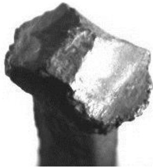
Fig. 108. Cut clasp nail circa 1855 showing the development of the clasp 'wings'. Author
