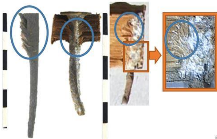
Fig. 23. Crushing and deflection of timber fibres in Baltic pine from cut floor brad 1887, Stringybark shingle circa 1843, and Hoop pine tiling battens showing deflection of timber fibres and secondary effects of zinc corrosion. Author
