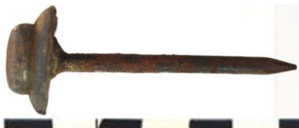
Fig. 148. Pirate copy of Stokes lead head roofing nail. A few copies were marked "WATERPROOF". Author.
