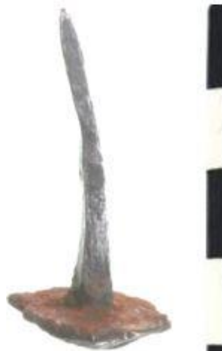
Fig. 91. A cast faceted head with a forged shank, shown in its casting position. Author.
