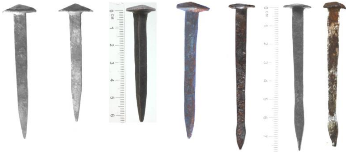
Fig. 29. L to R; two sizes of gate nails from the Naish collection, Salisbury, with a stout gate nail from Woolmers Tasmania 1828. An Essex Hurdle and a Kent 'Fine' Hurdle nail (both from Naish) and an 1880 Sussex Hurdle nail from Marden, Sussex. Last is a 1732 rafter nail, Bowlsh House, Darshill. Author
