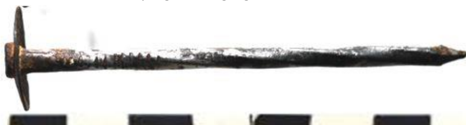
Fig. 149. Evenden disc head later version 48 Hopetoun Road, Warrnambool, with a spiral shank. Author.
