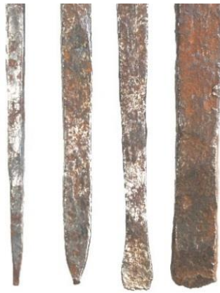
Fig. 27. Sharp, Spear, Spoon and Chisel points. Author
