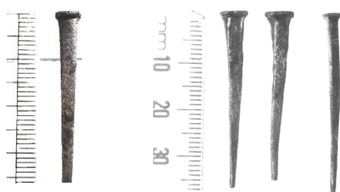
Fig. 102. Cut shingle brads and a lining nail found in Victoria of probable British manufacture. Author
