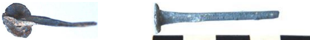
Fig.78. Spindly zinc slate nail circa 1843, Meredith, Victoria. (LEFT), and 1856 version, Warrnambool, Victoria, (RIGHT). Author.
