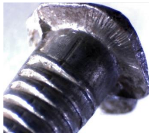
Fig. 142. Opposed clamping on an 1890 wire nail. Note how the teeth marks are impressed over the dressing score. Author
