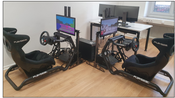
Figure 2: Test rig including steering wheels, pedals, seats and screens.
