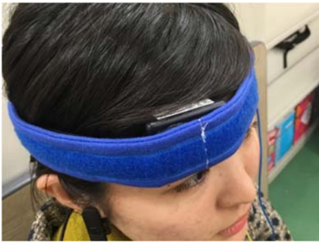
Figure 2: The HEG sensor and its installation.
