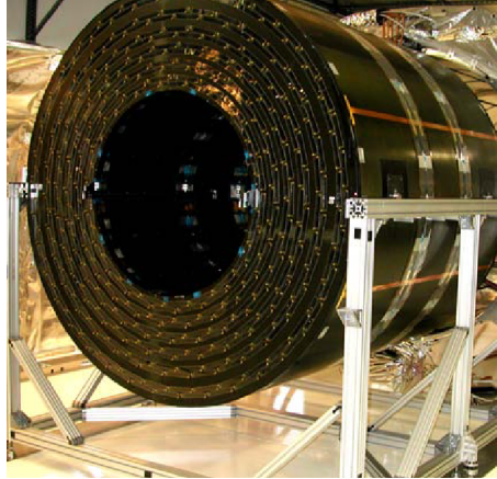
Figure 3.7. | The picture of the naked TOB wheel [20].
