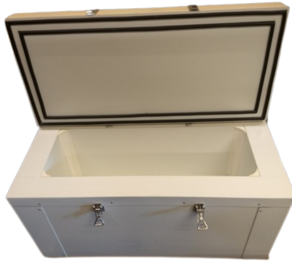
Figure 5.41. | Prototype cold box being assembled in Louvain la Neuve. The door has been removed and is resting on top. The opening will eventually be in the front.
