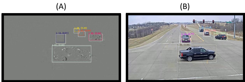
Fig. 4.6 Visual results on residual frames (A) versus raw frames (B) in Experiment 2. White bounding boxes represent the ground truth annotations, colored boxes represent the detections together with their respective IDs and confidence score.
