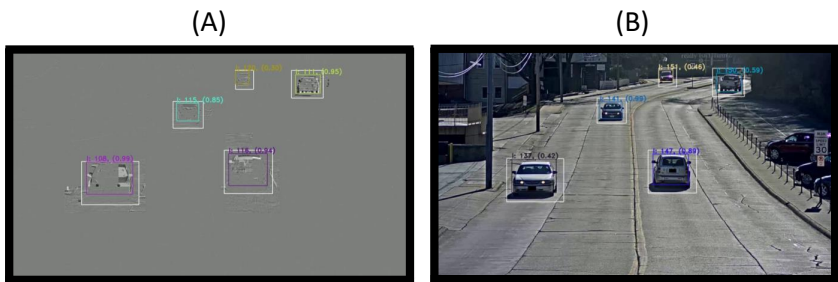
Fig. 4.5 Visual results on residual frames (A) versus raw frames (B) in Experiment 1. White bounding boxes represent the ground truth annotations, colored boxes represent the detections together with their respective IDs and confidence score.
