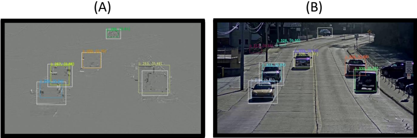
Fig. 4.7 Visual results on residual frames (A) versus raw frames (B) showing false positives in the background and foreground of the raw frame and detection mergers in the residual frame.
