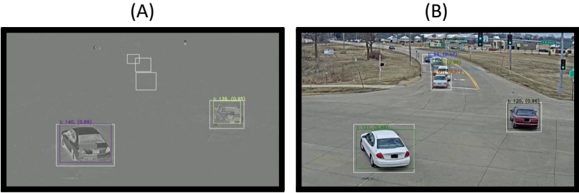
Fig. 4.9 Visual results on residual frames (A) versus raw frames (B) showing false negatives in residual frames when cars are stopped.
