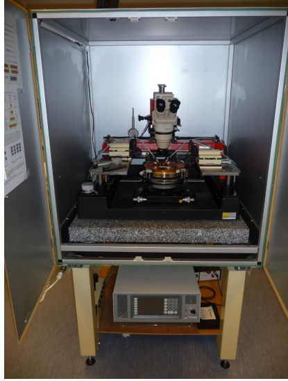
Fig. 5.6: On-wafer probing with Temptronics High Temperature control station.
