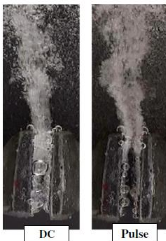
Fig. 23. Oxygen and hydrogen bubbles being produced simultaneously on a different nickel electrode immersed in a KOH solution with an electrode distance of 2 mm, E_{\text{on}} = 4.0 V, and E_{\text{off}} = 0 V. Adapted from [174].
