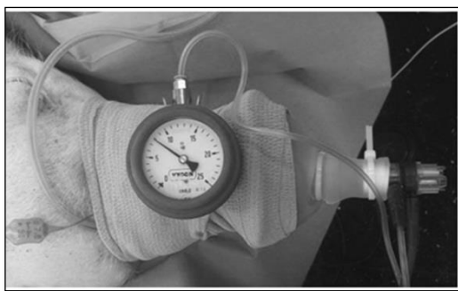
Fig.1: Experimental ventilation interface. The mask was adapted using an elastic strip to cover their labial commissure and limit air leaks.
