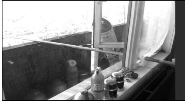
Fig. 46: Exhaled gas scavenger; Gas evacuation outside the room.
