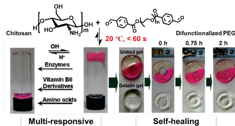
Figure 2.24. The multi-responsive and self-healing SCN hydrogels based on imine bonds formed by the chitosan and a dibenzaldehyde-terminated PEG. [180]
