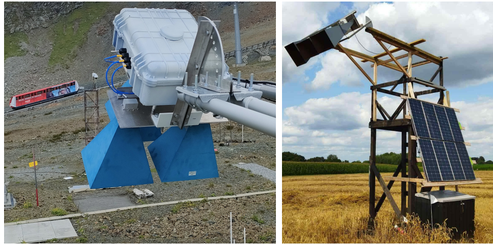
Figure 2. Field installation of the two radar systems showing two potential applications. The left tower, equipped with smaller horn antennas, operates in the C-band and is powered from the grid. The focus of this setup lies in measuring the soil–snow profile. This radar was installed during the summer at Weissfluhjoch, Switzerland, when the site was free of snow. The right tower, located in at Louvain-la-Neuve, Belgium, fitted with larger horn antennas, operates in the L-band and is supplied by a solar-powered battery system. Measurements performed at this location focus on the soil–vegetation profile.
