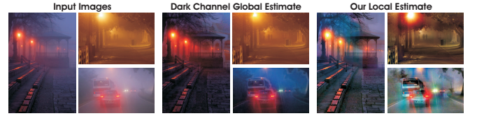
Fig. 2. Rough dehazing of night-time scenes. Designed for day-time dehazing, the well-known dark channel [16] has important limitations on night scenes because it uniformly estimates the airlight constant. As may be observed, our patch-based estimate (also not refined) of the airlight component is more appropriate for the night-time hazy scenes. In particular, color and details that are close to light sources are better enhanced. By simply replacing these estimates in the model equation results in some rough dehazing outputs.
