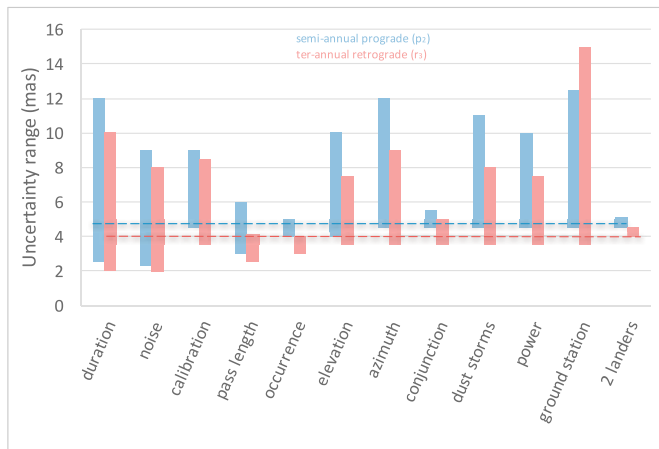
Fig. 28. Levels of improvement and degradation in the nutation determination for the different cases tested in this study. Nominal uncertainties in p_2 and r_3 correspond to dashed-horizontal blue and red lines, respectively. (For interpretation of the references to color in this figure legend, the reader is referred to the Web version of this article).
