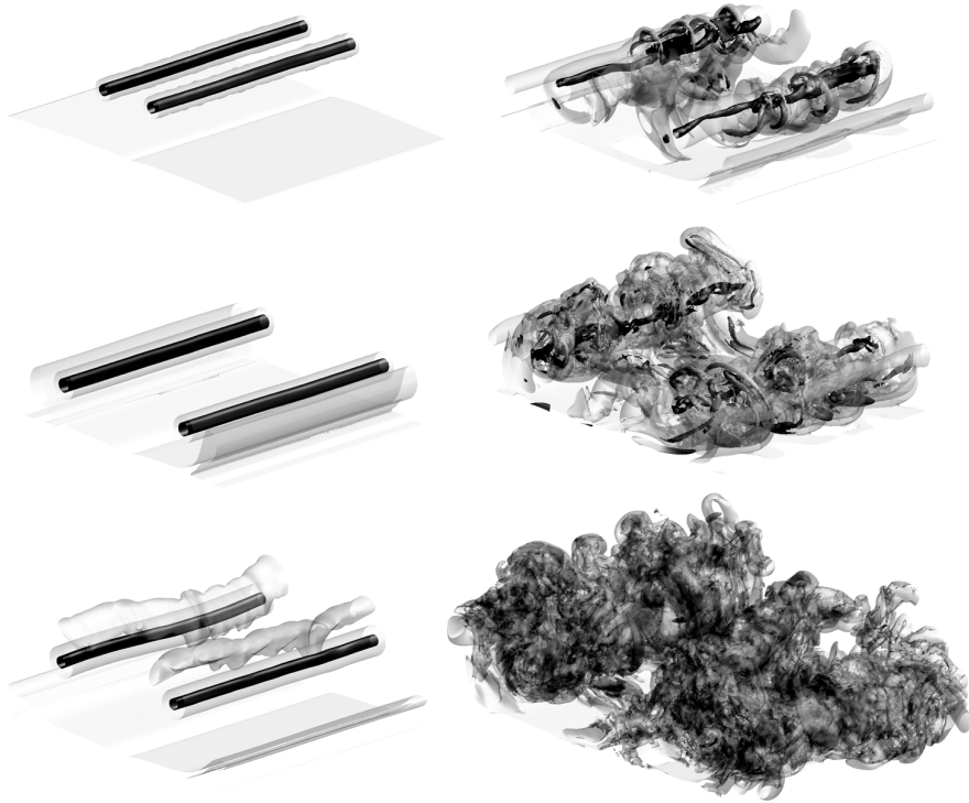
Figure 1.17: Two vortex system in ground effect at Re = 5000 : two isosurfaces of vorticity are shown (for one periodicity length): \|\omega\|b_0^2/\Gamma_0 = 10.0 (opaque) and 1.0 (semi-transparent). The grey scale is proportional to \omega_x . Times shown are: \tau = 0.08 ; \tau = 1.6 (secondary vortices emanate from the ground); \tau = 2.9 (short-wave instabilities visible on the secondary vortices); \tau = 3.5 and \tau = 4.2 (strong interactions between the vortices); \tau = 6.1 ("turbulent" and decay phase).
