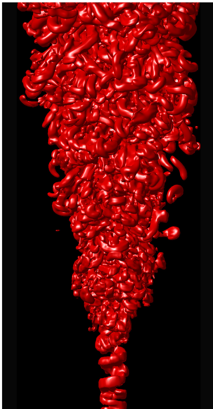
Figure 5.2: Round jet at Re = 10000 : 3-D view at t/t_0 = 495 . One isosurface of \lambda_2 = 0 is shown at half the grid resolution.
