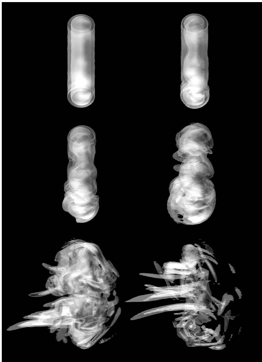
Figure 1.13: Vortex ring at Re = 5500 : 3-D side view of the instabilities. The same isosurfaces of vorticity are shown.
