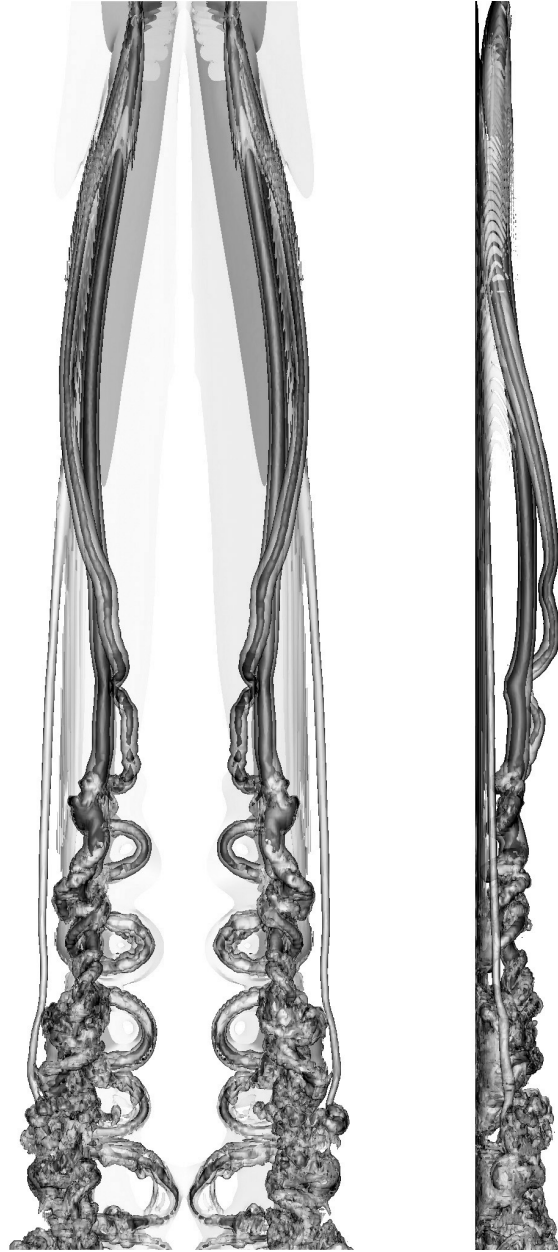
Figure 1.20: 3-D Space developing LES of wake vortices behind an elliptically loaded wing in ground effect: isosurfaces of vorticity norm, ||\omega|| t_0 = 80 (opaque) and 25 (semi-transparent), colored by the longitudinal component of vorticity, when the flow has reached it's regime. Top and side views.
