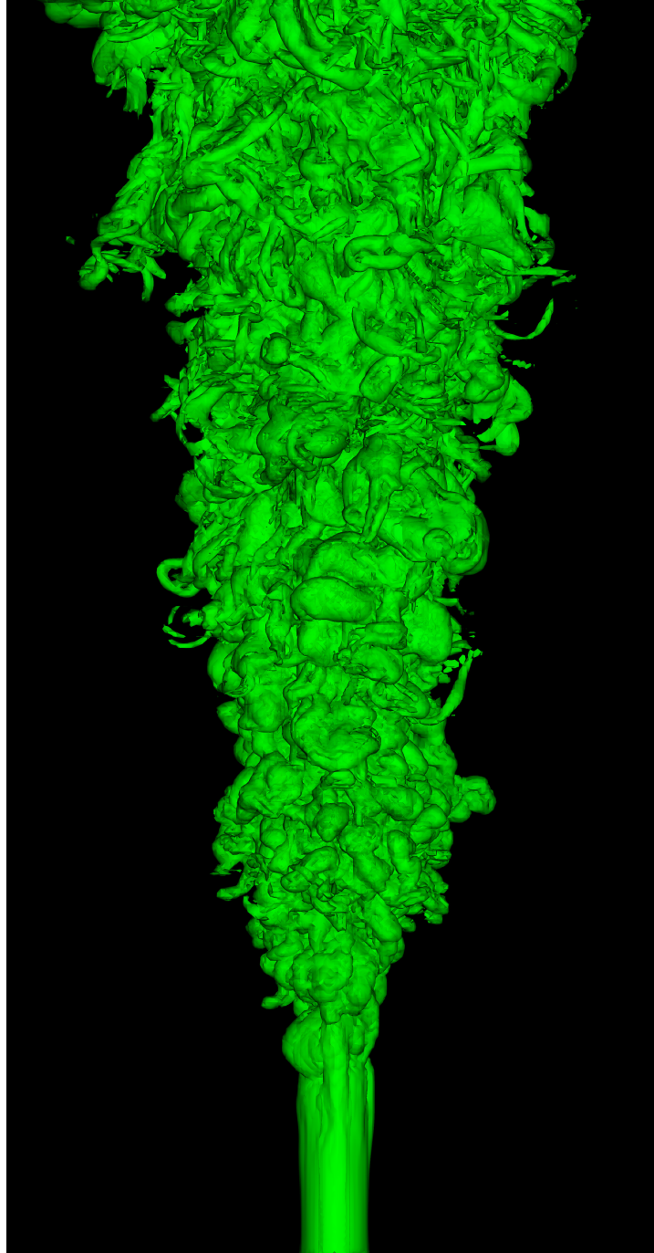
Figure 5.1: Round jet at Re = 10000 : 3-D view at t/t_0 = 495 . One isosurface of vorticity is shown ( \|\omega\|t_0 = 0.2 ) at half the grid resolution.
