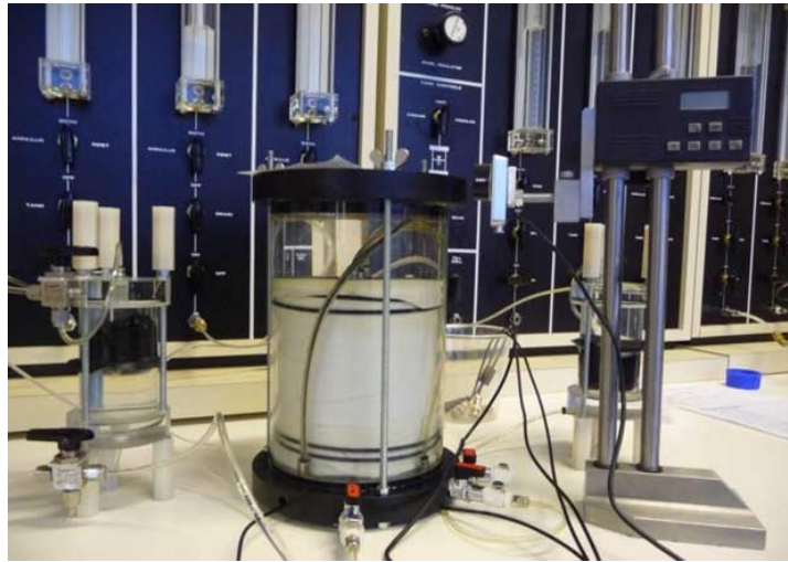
Figure 1. Flexible-wall hydraulic conductivity cell provided with bender elements and a cathetometer.
