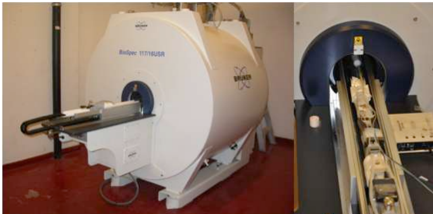
Figure 1. The 11.7T MRI machine dedicated to small animal applications (Biospec, Bruker, Ettlingen, Germany) and representative picture showing the small animal setup.
