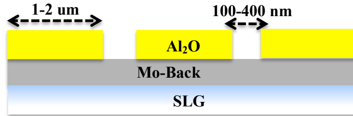
Figure 6.1: Schematic of the rear point contact design
