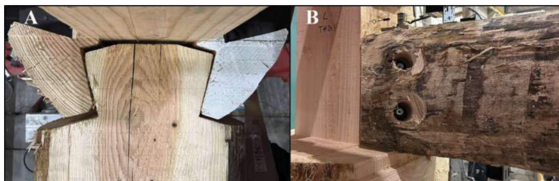
Figure 2: (A) Top view of dovetail joint slotted into a whole log column element. (B) Whole log beam seated at the tenon on the column support and fastened to the column centre with structural screws and material volume removed below beam for access purposes.
