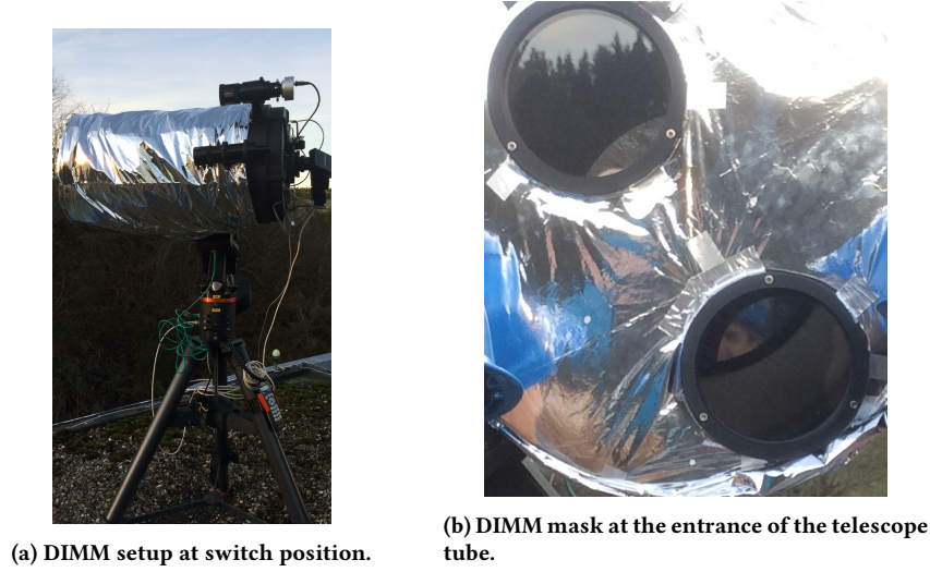
Figure 6.8 – Illustration of the DIMM used at Redu in the framework of SALTO. [Qua+23]
