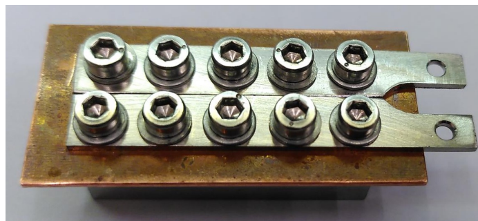
Figure 4.16: Picture of the straight "blades" mounted on the multichannel block, with a copper piece for the sealing.
