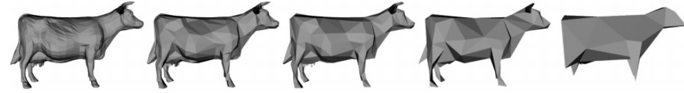
Figure 5.2 Edge deletion in a mesh simplification. The edge V_1 V_2 is replaced by the vertex \bar{V} which is connected to all the neighbors of V_1 and V_2 . Image courtesy [94].
