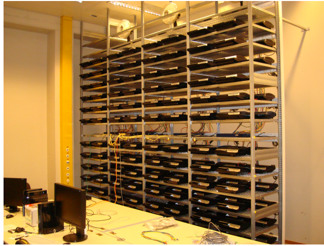
Figure 1.1: The cluster of 214 PlayStation 3 consoles of the Laboratory for Cryptologic Algorithms of EPFL.
