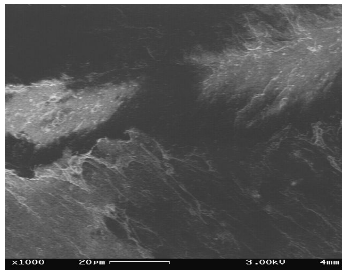
Figure 4.52.: SEM picture of the sample NQ24 cross-section (PU series A with 1wt% CNT), under a 3kV electric field. The little white dots are most probably CNTs or pieces of CNTs, they are regrouped in agglomerates and there are volumes of material devoid of CNTs (dark areas).
