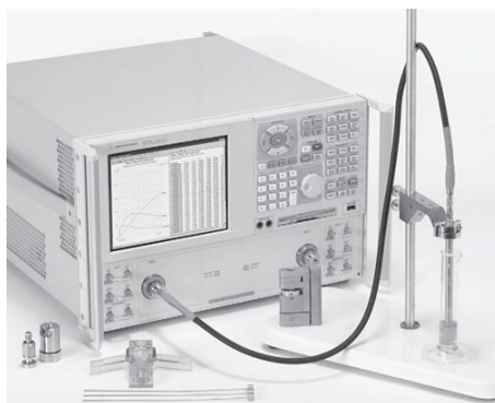
Figure 6.5.: Picture of the dielectric probe kit, not connected to our PNA-X but to similar equipment, from its user manual.
