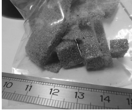
Figure 3.32.: Picture of the low-density flexible PU based foam containing 0.35 wt% of CNTs fabricated at CSIC, the homogeneous grey colour of the sample is usually the sign of a good dispersion of the CNTs.
