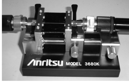
Figure 3.13.: MUT used as substrate in a microstrip TL fitted in an Anritsu model 3680K sample holder, to be connected to a VNA.
