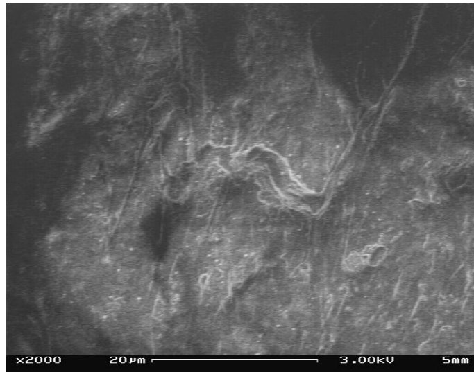
Figure 4.53.: SEM picture of the sample NQ29 cross-section (PU series A with 2wt% CNT), under a 3kV electric field. The little white dots are most probably CNTs or pieces of CNTs, there are volumes of material devoid of CNTs (dark areas).
