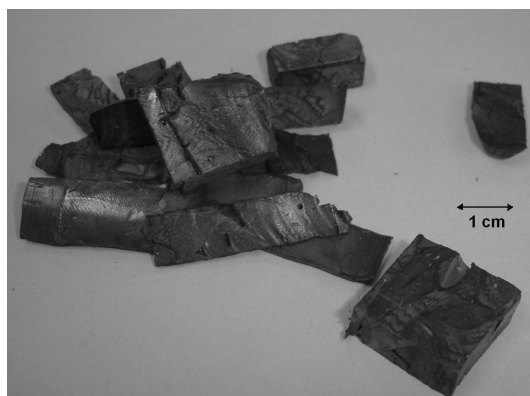
Figure 5.7.: Picture of a nanocomposite foamed sample, PCL matrix with 2 wt% CNT content (already cut into pieces in preparation prior to its characterization).
