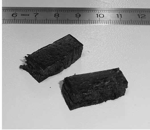
Figure 3.35.: Picture of the rigid PP based foam containing 8 wt% of CNTs fabricated at ULg, the very dark colour of the sample hinting at a high electrical conductivity of the sample.
