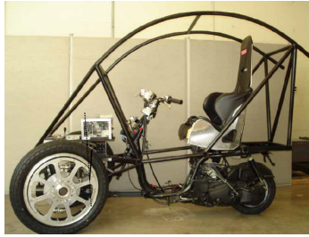
Figure A.14: Research NTV prototype developed by Kidane at the University of Minnesota [54].
