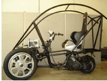
Figure 2.14: Research NTV prototype developed by Kidane at the University of Minnesota [54].
