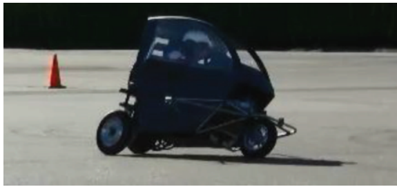
Figure 2.8: The prototype NTV developed by Equos working based on a FTC actuation [32].
