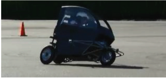
Figure A.30: The prototype NTV developed by Equos working based on a FTC principle [32].
