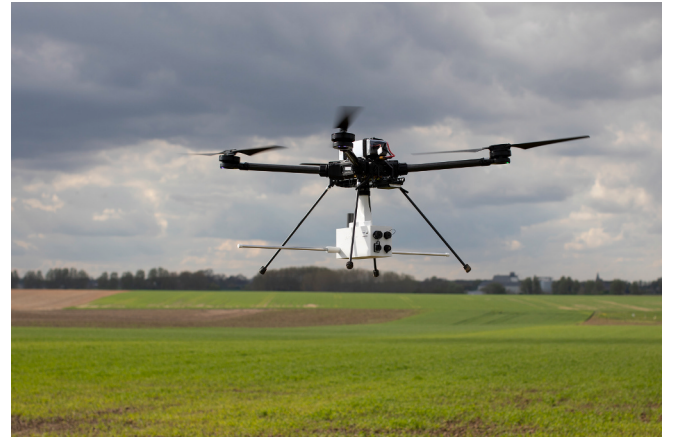
Fig. 2. Drone-borne mapping of root-zone soil moisture on the test site using the gprSense® system ( www.gprsense.com ), mounted on a Tundra drone from Hexadrome (Saint-Ferréol-d'Auroure, France). The photograph shows the 2024 version of the instrument, while the data presented in this study were collected with an earlier 2023 version. The gentle slope toward the talweg is visible in the background.
