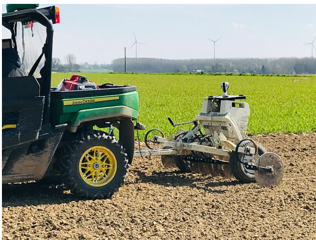
Fig. 3. Mapping soil electrical conductivity using Electrical Resistivity Tomography (ERT) with the Veris Q2800 system (Veris Technologies, Salina, KS, USA) towed by an all-terrain vehicle (ATV). The system provides measurements at two depths: 30 cm and 90 cm.
