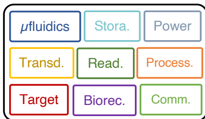
Fig. 1.6 Schematic representation of a generic biosensor architecture, describing the sensor in terms of its necessary functional blocks to reach the biosensing functionalities. The required functional blocks include the microfluidics, the transducer, the bioreceptors, the readout and processing system, the data storage capacity and communication, and possible power supply.
