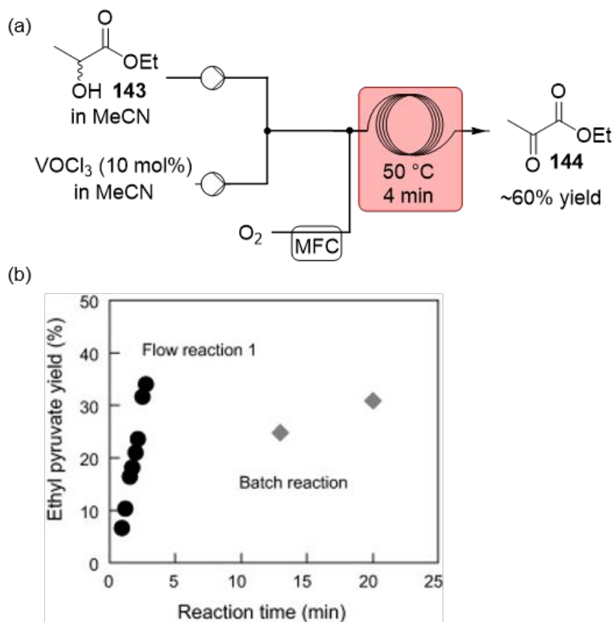
Figure 101. (a) Oxidation of ethyl lactate in ethyl pyruvate using \text{VOCl}_3 as the catalyst. 795 (b) Yield of ethyl pyruvate as a function of the reaction time for the batch and flow aerobic oxidation of ethyl lactate catalyzed by \text{VOCl}_3 . Reproduced with permission from ref 795. Copyright 2011 Elsevier.
