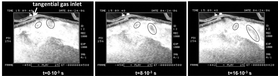
Fig. 8. High speed CCD camera observations at 1000 frames/s visualizing the formation and motion of bubbles through a bed of 300 \mu\text{m} alumina particles rotating in a vortex chamber. Vortex chamber design as in Fig. 2; camera focusing on a single gas inlet slot. Total gas flow rate: 0.2 \text{m}^3/\text{s} , solids loading: 1.1 kg, bed rotating at 3.5 rps (10G). (Adapted from Ref. [20]).
