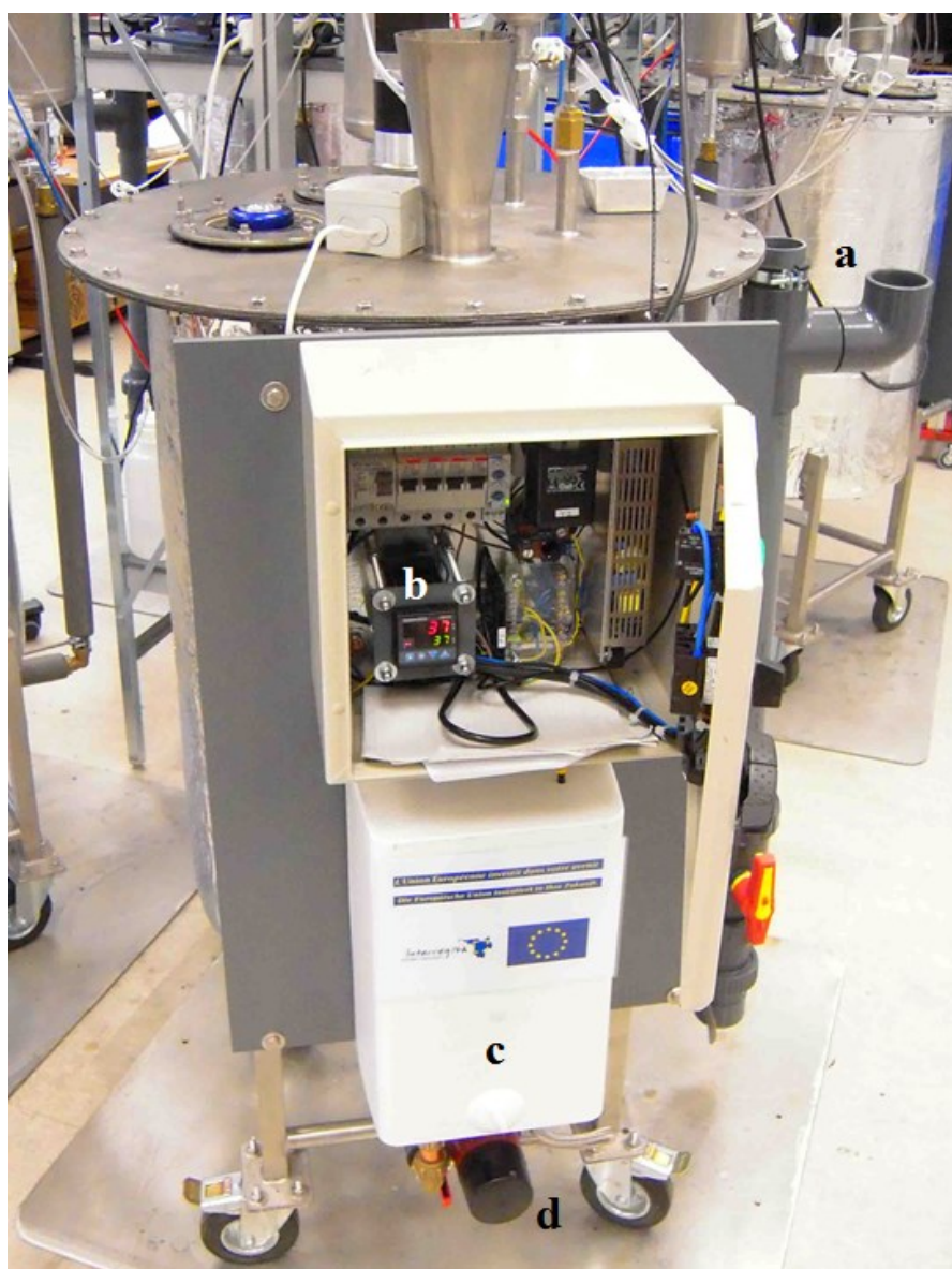
Figure A 2. One of the four 100-L continuously stirred tank reactor developed for this research: (a) lateral overflow pipe; (b) proportional-integrative-derivative temperature controller; (c) electric boiler; (d) circulation pump.
