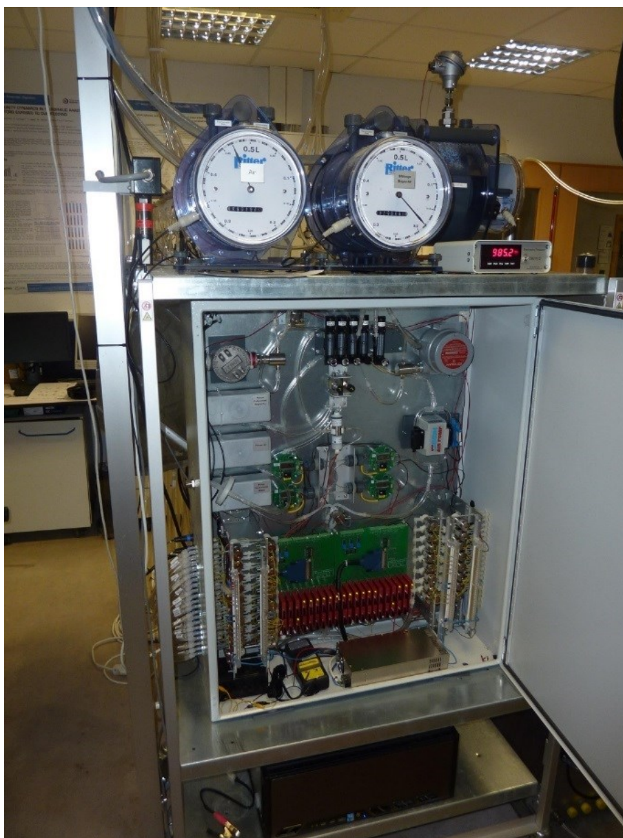
Figure A 8. Main unit of the biogas monitoring system N° 2 developed in the framework of this research.
