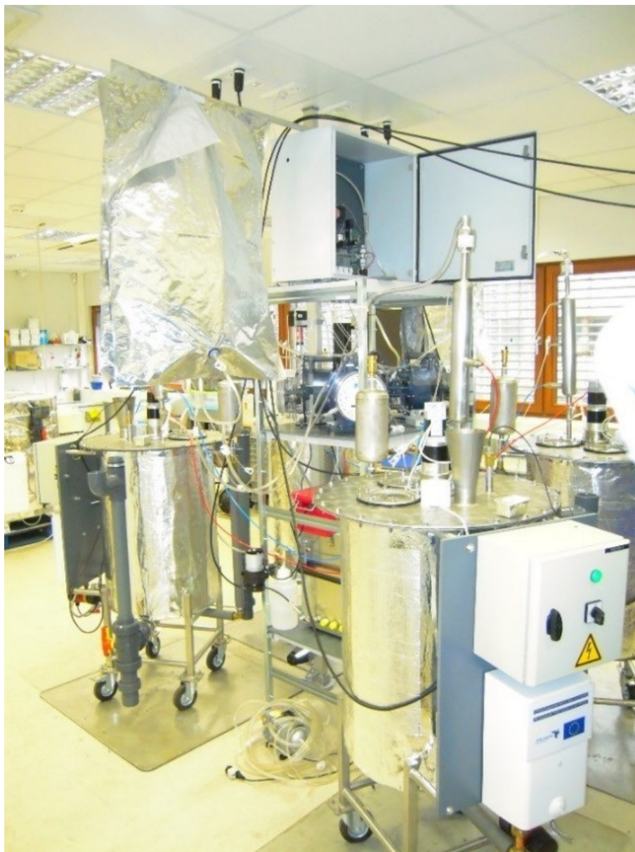
Figure A 4. Biogas monitoring system N° 1 developed in the framework of this research (the system is placed in centred position among the four 100L continuously stirred tank reactors).
