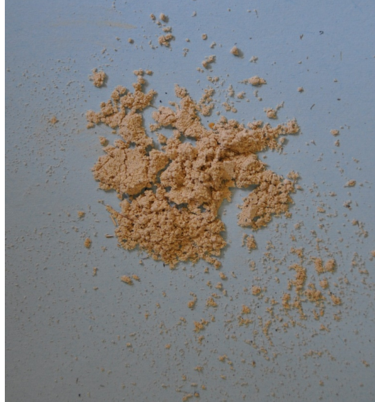
Figure 8.11: Powder produced in during spray drying exp. 8 with the spray nozzle mounted outside the dual-zone vortex chamber. Vortex chamber design and operating conditions: see Table 8.1.
