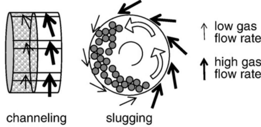
Figure 2.10: Schematic representation of channelling and slugging in vortex chambers [62].
