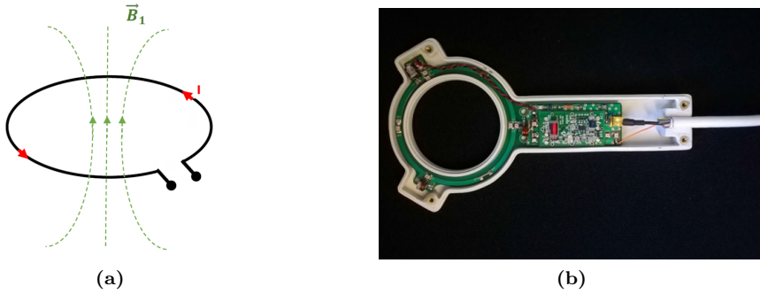
Figure 1.9: (a) Surface loop coil and the orientation of its magnetic field [18]. (b) Surface loop coil used in the Rx mode with its preamplifier [19].
