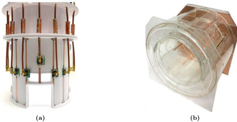
Figure 1.27: (a) Dipole and (b) monopole antenna arrays for the human head imaging at 10.5T [41], [40].
