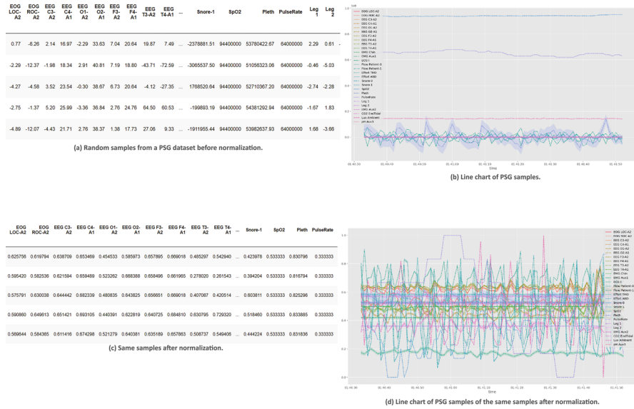
Fig. 7 The effect of Min-max normalization on PSG samples and visualization: (a) is a random snippet from a PSG dataset before Min-max normalization, (b) the line chart of the same snippet, (c) the same set of samples after min-max normalization, and (d) shows that all channels are on the same scale
