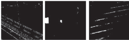
Fig. 12: Distortion of test videos: improper chroma component, blocking effects and improper interlacing.
