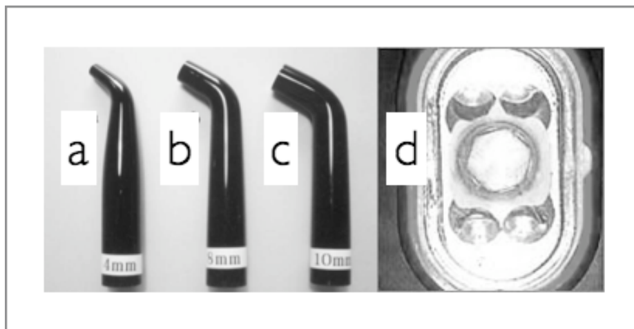
Figure 5 - Different light guides available; a) and b) are turbo tips, c) is the regular light guide and d) presents the diodes directly behind a simple transparent cover.
